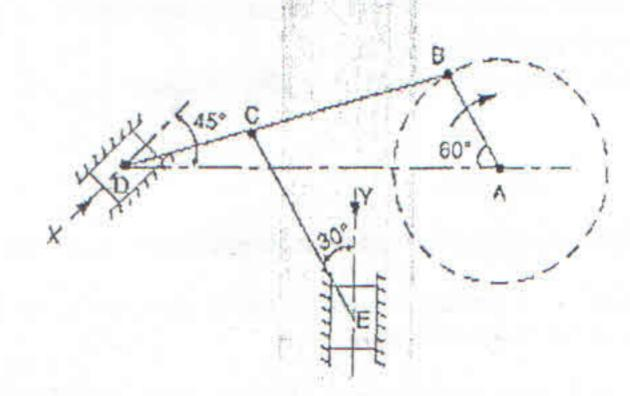
The crank AB turns uniformly at 180 rpm in the clockwise direction and the blocks at D and E are working in frictionless guides. Draw the velocity diagram for the mechanism and find the velocities of the sliders D and E in their guides.
